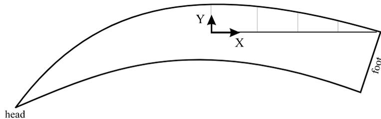
As with the Depth curve in the headsail/mainsail program, the more curvature there is in this curve, the more shape there will be in the panels in that region. Making this curve fuller will have the effect of pushing the foot aft and hence increasing the amount of shape in all the panels in the lower half of the sail.
