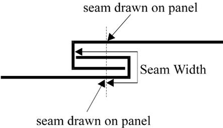
If **Seam on both sides** is not ticked, the overlap is simply the **Seam Width** :
