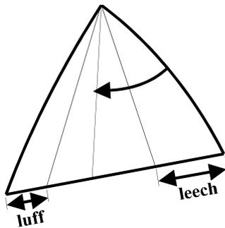
**leech** : Edge width of the leech panel. This does not include the seam allowance or shaping.
