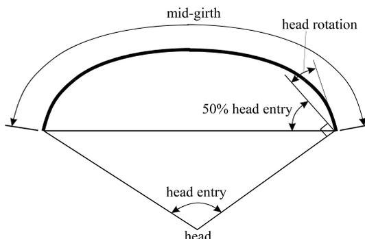
In the case of the head-chord, the entry angle is the same as the mid-chord except the girth is of course equal to zero. Although its girth is zero, the shape of the head-chord influences the area between the mid-chord and the head.
