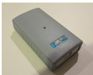
With the ProSail plotter mkIII or the ProSail digitiser, the dongle is an optional extra and is not supplied as standard. With these machines the software will run so long as the USB cable from the "USB to Serial converter" is plugged into the computer (the machine does not need to be turned on, just the USB cable plugged in to the computer).
