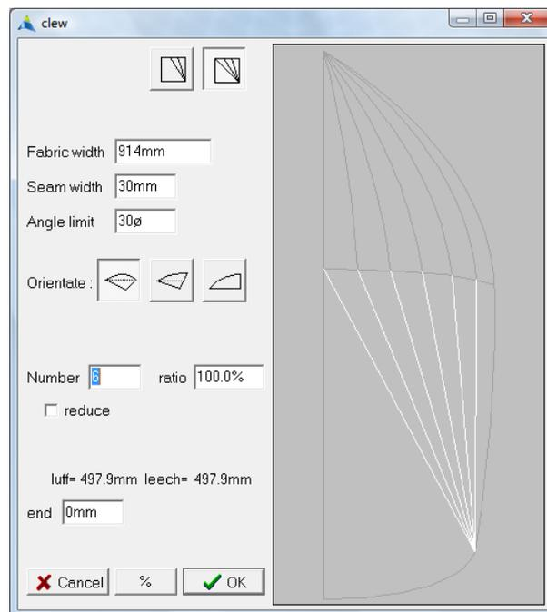
To make these panel seams line up with the seams above, use the same **Number** and **ratio** as the panels above.
