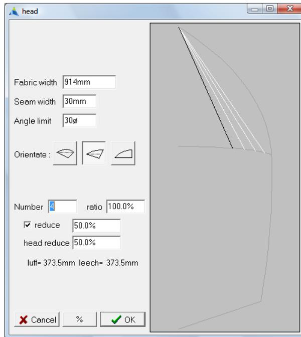
**Reduce** splits the head panels into regions. The value specified for **reduce** is the length of the region either as a % of the horizontal interface seam or in absolute length. As well as specifying a value for reduce, you can also click on the end of this reducing line and drag it to the required location along the horizontal interface.
