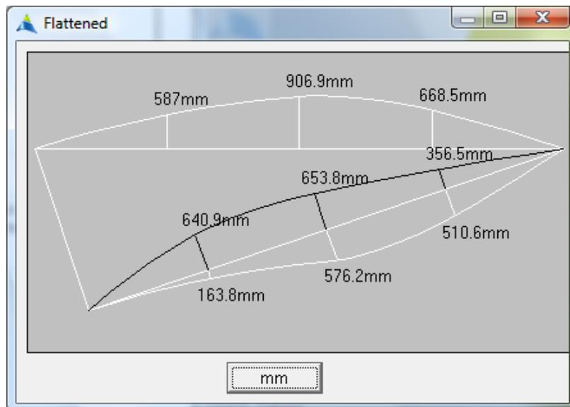
This outline is the conventional flattened spinnaker (that most people are familiar with) produced by folding the spinnaker down the centre seam and pinning it out as flat as possible on the floor. This is similar to the Flattened method in the ProSail (headsail/mainsail) program except of course it only looks at half the sail.
