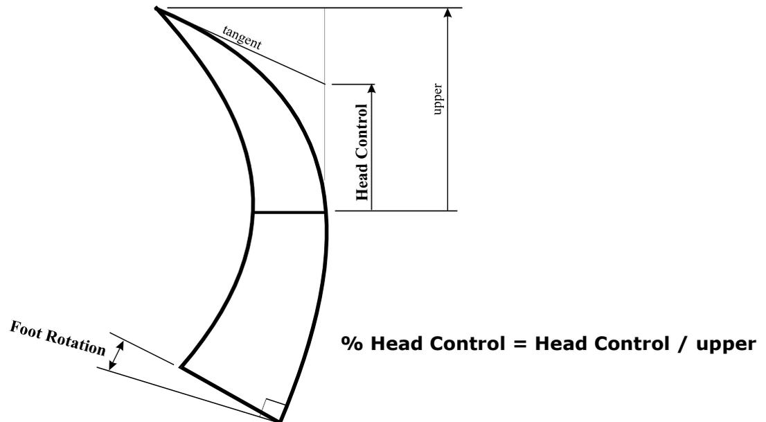
**Head Control** This is very important and controls how flat the head is. Increasing **Head Control** will increase the fullness in the head. It is very important not to make **Head Control** too large. Remember that the flying sail will lift and so the picture on the screen should have significantly lower shoulders than the flying shape. A typical value is 55%. Larger values may result in the head folding. If in doubt specify a lower **Head Control**.
