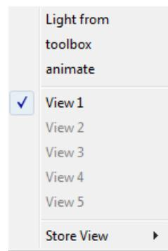
**Light from :** Click on this to animate the direction of the light source. Works in a similar way to animating the view except it displays 2 arrows indicating the direction of the light source. The arrows are largest when pointing directly into the screen and change colour when at 90 degrees to this direction.
