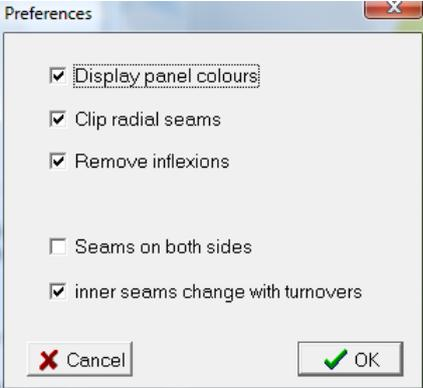
If **Seam on both sides** is ticked, the seam can be joined as follows where the **Seam Width** entered in the panel dialogues is 1.5 times the the size of the overlap :
