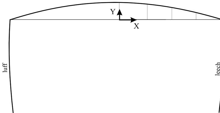
This shape is added to the bottom of the foot panel after panel development. See the note on **Foot Rotation** in the Dimensions chapter.
