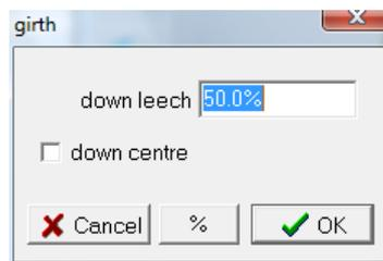
Enter the desired location down the leech. This will calculate the shortest distance from this leech location to the centre seam. This will be half the girth across the sail at that location. To generate a girth from a leech location to a location down the centre seam, tick **down centre** and enter a value.
