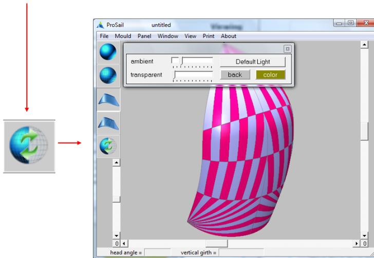
The view direction can be changed by dragging any of the 3 scroll bars around.
