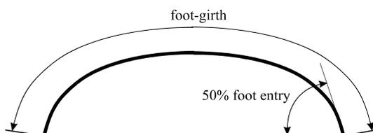
As well as the girths and entry angles which are defined by the **Dimensions** dialogue, the shape of each chord can be further defined using arcs. The number of arcs is determined by **Chord Sectors** in the **Dimensions** dialogue. If **Chord Sectors** is set at 2 (recommended) the follow geometry defines a chord (half of a chord for symmetry) made up of 2 arcs :
