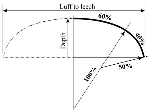
**length** defines the % of the chord girth each arc covers. In this case the inner arc covers 60% of the chord girth and the outer arc covers 40%.
