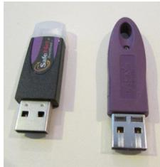
A dongle is a small USB connector that plugs into a USB port on your computer. For many ProSail machines, a dongle is required for the software to run.
