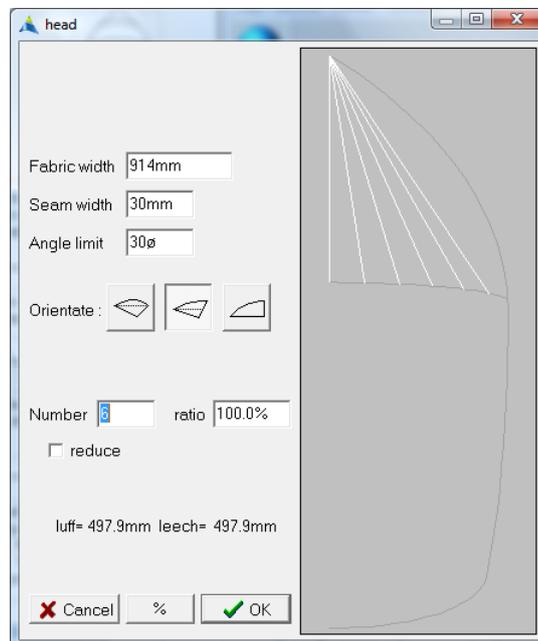
All radial-head panels are shaped on both sides. They are however not symmetrical and are of different lengths. The radial head dialogue operates the same as for headsails and mainsails except it only displays half of the head panels.
