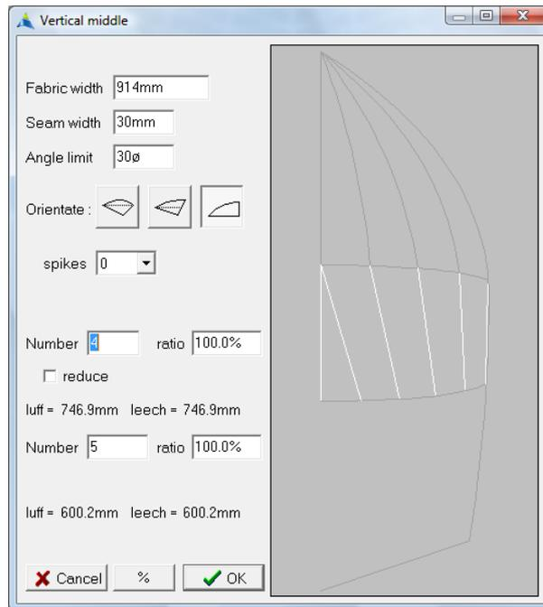
Vertical panels in the middle of the sail are specified using two sets of **Number** and **ratio** :
