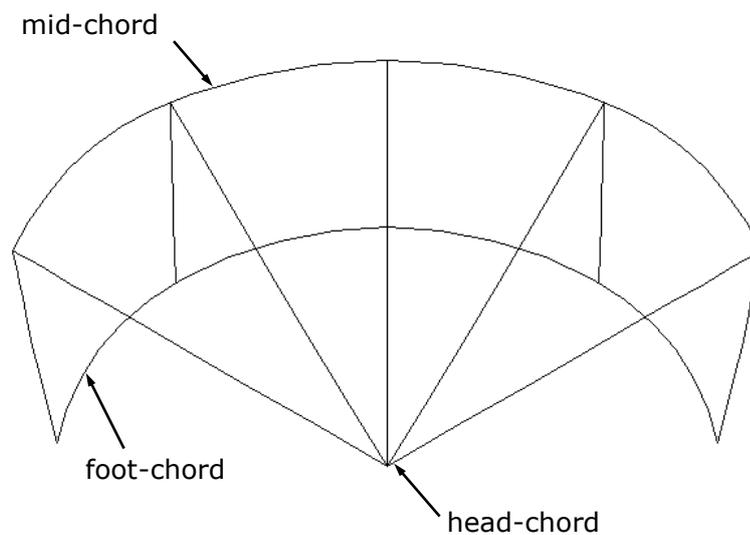
Before entering the Chord window, some of the dimensions entered in the **Dimensions** dialogue already partially define the shape of the chords. For the mid-chord, the girth is equal to **Mid. Girth**. The entry angle of the chord is equal to the **Head Rotation** + half the **Head Entry** :
