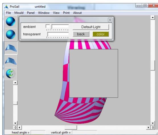
There are two animation modes when moving the mouse horizontally. It will either rotate the view in a horizontal plane or it will tilt the view clockwise/anticlockwise. To toggle between these 2 modes, press and release the Ctrl key on the keyboard while animating. This will redisplay the square outline. After moving the mouse into this square again, the mode will have changed.
