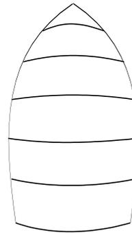
These panels are developed from the bottom of the sail up to the head. Since this is the opposite direction from normal, the panels are shaped on their bottom edge and straight on the top.
